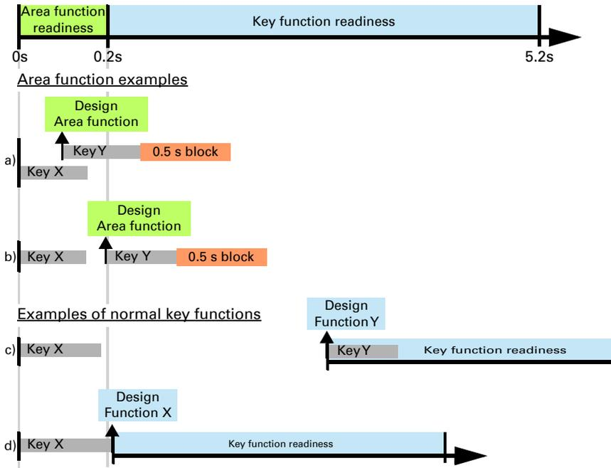
If the area function in the ETS is disabled, the keys can be used normally at any time.
