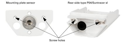
The holes in the lower part of the housing must be carefully broken out for the screw fastening. The lower part of the housing is screwed together with the sensor mounting plate from the inside.
