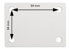
Fig. 2 Hole diameter 6.2 mm
