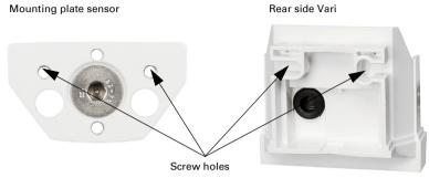
The holes in the lower part of the housing must be carefully broken out for the screw fastening. The lower part of the housing is screwed together with the sensor mounting plate from the inside.
