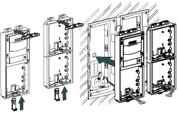
**3** Fix the assemblies to the flush-mount boxes with screws.
