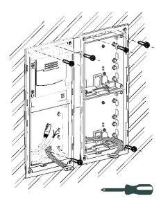
Make the connections of the basic unit and prepare the additional modules. Pass the bus cables through the gaps.
