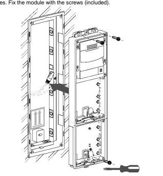
3 Connect the cables to the basic unit and interconnect the additional modules with the bus as shown in the schema.
