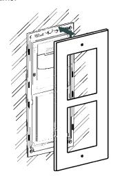
**6** Fix the frame by using the supplied Allen key.
