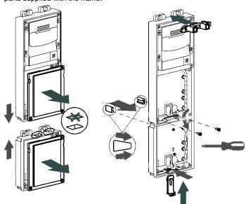
2 Place the assembly inside the flush-mount box and recover the cables. Fix the module with the screws (included).
