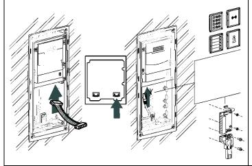
4. Fix the blind panel (or additional modules that remain in sight) with the supplied screws and put the labels with captions next to the buttons.
