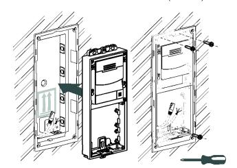
3 Connect the cables to the basic unit and interconnect the additional modules with the bus.
