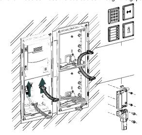
**5** Interconnect the additional modules with the bus as indicated in the schema and then, fix the additional modules with the supplied screws.
