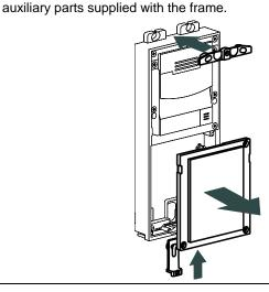
Place the basic unit inside the flush-mount box and recover the cables. Fix the enclosure with the screws (included).
