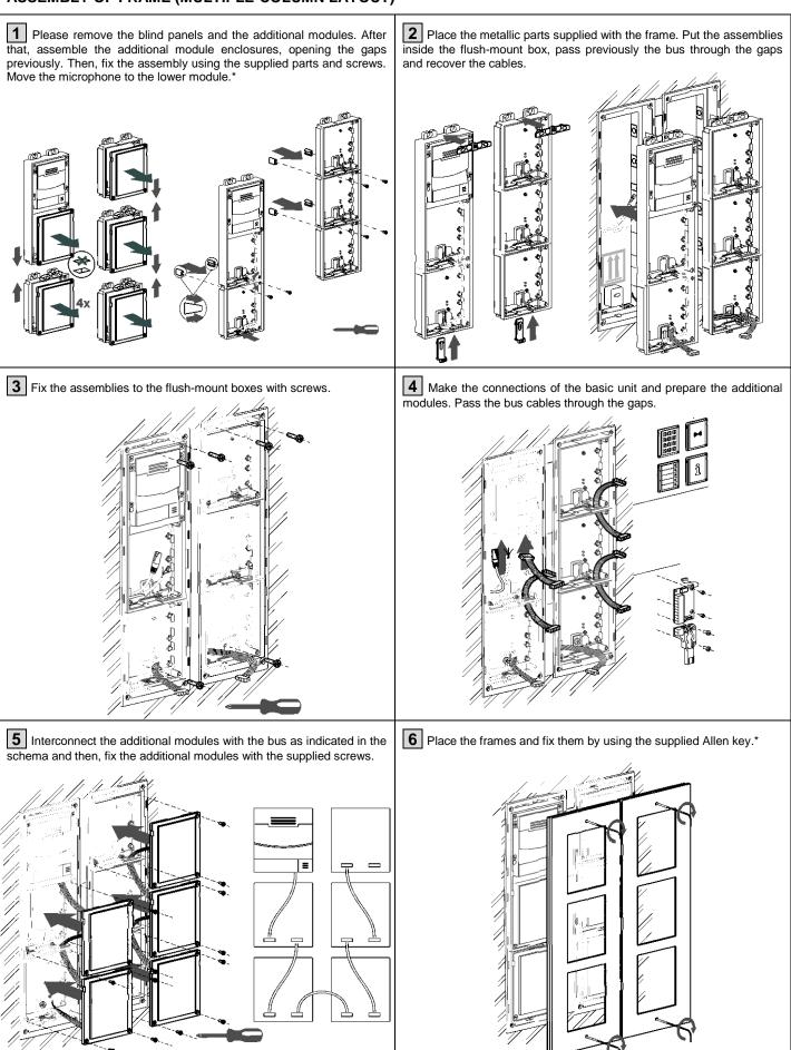
\*In case of acoustic deficiencies, Zennio may supply a modified frame for whose installation step number 1 should be ignored. In such case, though, it is essential that the microphone remains properly connected.
