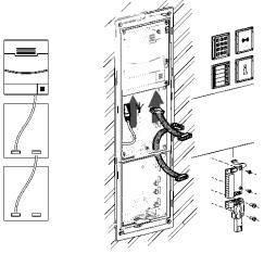
4 Fix the blind panel (or additional modules that remain in sight) with the supplied screws and put the labels with captions next to the buttons.
