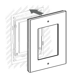
**6** Fix the frame by using the supplied Allen key.
