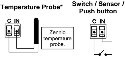
⚠ Commons of different devices must not be connected together.
