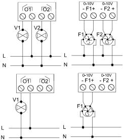
Figure 2: (From left to right and from up to down) Wiring examples for two valves, two fans, one valve and one fan.
