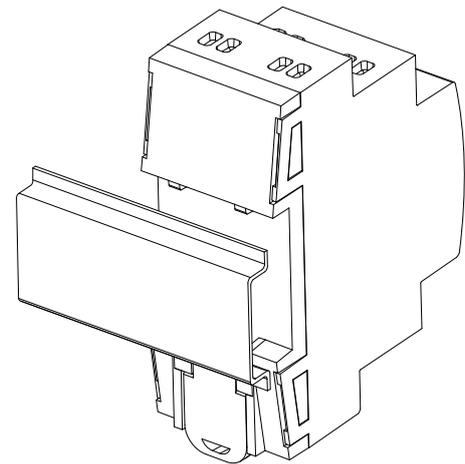
Figure 3: Mounting MINiBOX 40 v3 on DIN rail
