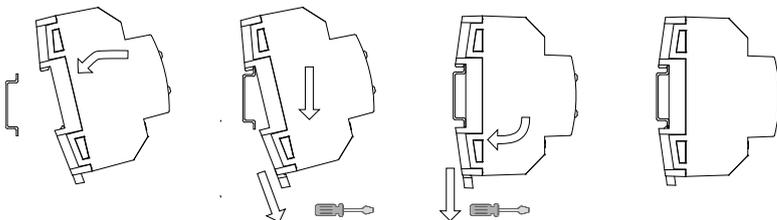
Removing MINiBOX 40 v3 from DIN rail:
