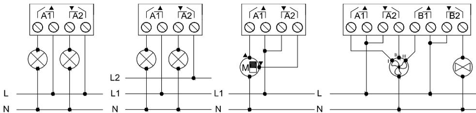
⚠ In order to ensure the expected status of the relays, please check that the device is connected to the KNX bus before energizing the power circuit.
