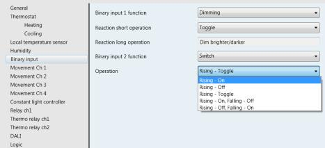
Figure 22 - Configuration options for binary switch input
