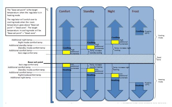
Figure 16 - Asymmetric regulator functionality
