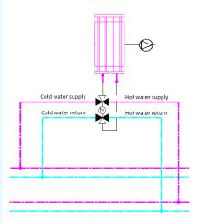
Figure 30 - 6-Way valve for combined heating and cooling control
