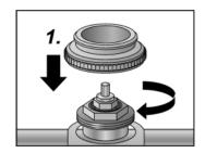
Screw the valve adapter manually onto the valve.
