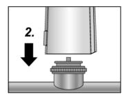
Position the OEM Actuator manually in vertical position to the valve adapter.
