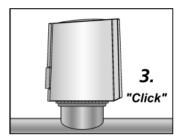
Latch the OEM Actuator to the valve adapter by manually applied vertical pressure; this can be done noiselessly and without any problems.
