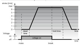
In case of the normally closed version, the valve is opened steadily by the ram motion upon switching on the operating voltage and after expiry of the dead time
