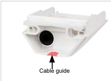
*b) If the power lead is to be surface-mounted, the cable guide is broken off. The lead is then fed into the device at the underside of the housing.*
