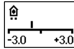
Fig. 6 Mode display with scale display and range. Shows the possible adjustment range (as set in the ETS). The control position in the image reads "Base target value reduced".
