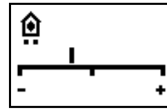
Fig. 4 Mode display with scale display for adjusting the base target value. The control position in the image reads "Base target value reduced".
