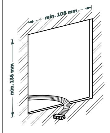
Place the box in the hole, recover the cables and fix the flush-mount box to the drywall by means of the screws that adjust the flaps to the drywall thickness. Please, pay attention to the top orientation mark.
