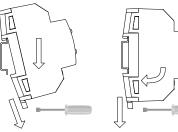
Removing MAXinBOX 24 v2 from DIN rail:
