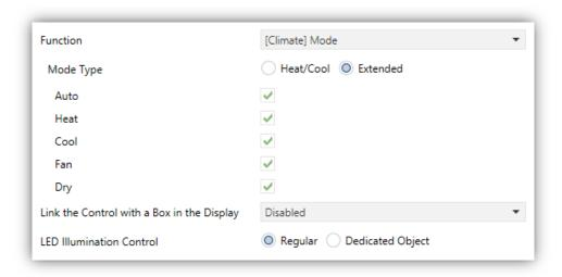
Figure 29. Individual Buttons – [Climate] Mode (Extended).
