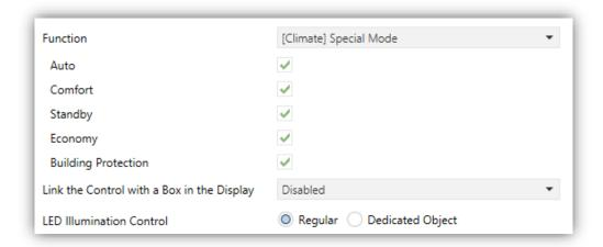
Figure 44. Pair Buttons - [Climate] Special Mode Control
