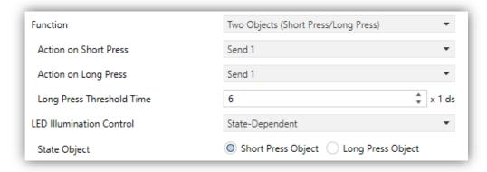
Figure 21. Individual Button - Two Objects (Short Press / Long Press).
