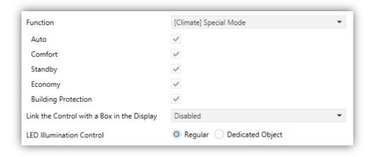
Figure 30. Individual Buttons - [Climate] Special Mode Control.
