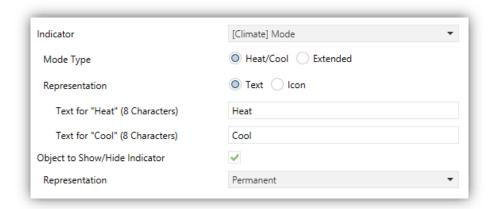
Figure 56. Display indicator – [Climate] Mode – Heat/Cool.
