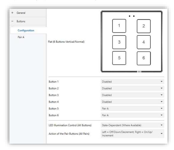
Figure 15 Buttons - Configuration
