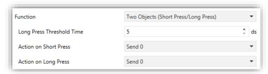
Figure 21 Individual Button - Two Objects (Short Press / Long Press).
