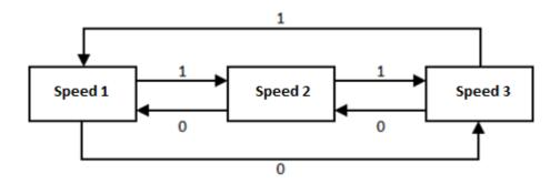
Figure 13. Cyclical fan step control (three fan speeds without automatic mode).
