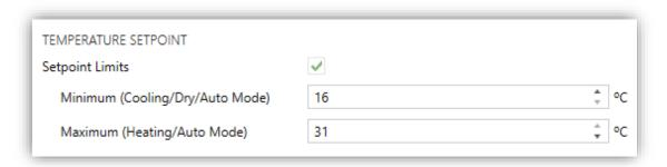
Figure 8. AC Gateway. Configuration. Temperature setpoint.
