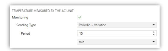
Figure 7. AC Gateway. Configuration. Temperature measured by the AC unit.
