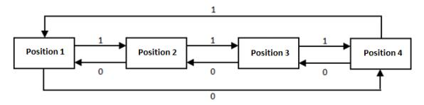
Figure 16. Cyclical flap step control (4 positions and no swing function)
