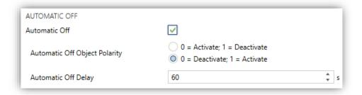
Figure 13. A/C Gateway. Configuration. Automatic off.
