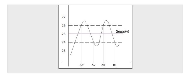
The main disadvantage of this algorithm, when compared to other advanced systems, is the permanent fluctuation around the setpoint temperature, which has a direct impact on the power consumption and on the comfort:
