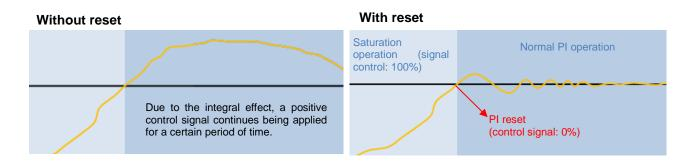
Figure 4. Effect of Resetting the Accumulated Integral Error after Signal Saturation.
