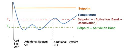
greater or equal than  $T_4$  (being  $T_4$  the sum of  $T_3$  plus the deactivation hysteresis).
