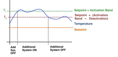
Figure 5. Switching the additional system on and off in cooling mode.
